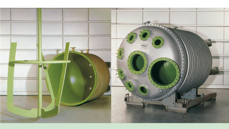
In the spraying sinter procedure (airless and compressed air process), Gutbrod works with Teflon® PTFE and Teflon® FEP. The coating is sprayed on and then "sintered" at 220° C to 420° C.
